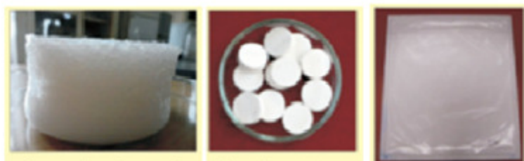
Superabsorbent Gel Drug in cassava from cassava starch Starch Biofilm from starch nanomatrix
