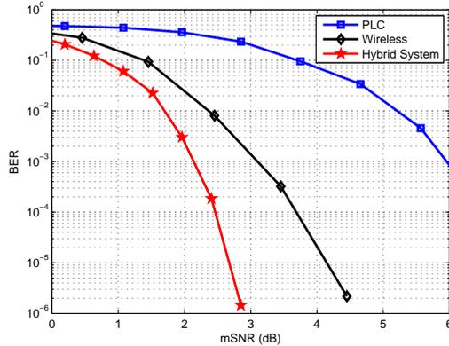
Fig. 7. Bit error rate versus multi-channel SNR.
