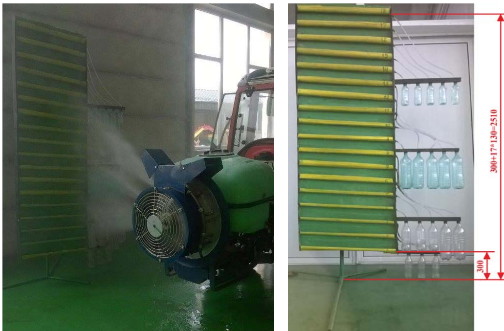
Figure 1 The laboratory stand for the dispersed solution distribution uniformity study of the vineyards TARAL 200 PITON TURBO spraying machine
