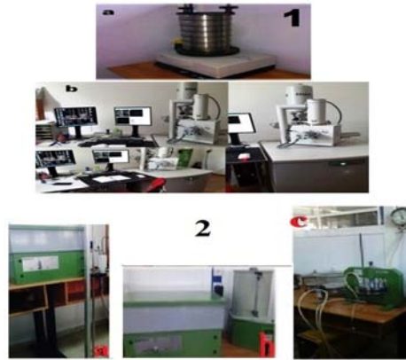
Figure 2 The tools used in research: 1: equipment used to analyze the morphology of mineral particles: a) shaker electromagnetic; b) equipment used in microscopic analysis SEM; 2: all equipment used in the study of hydraulic properties a) sandbox; b) sand/ kaolin box; c) pressure membrane apparatus
