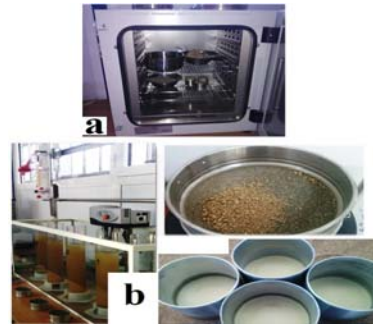
Figure 2 Equipment used to analyze the physical properties: a) drying machine b) Eijkelkamp Pipette Apparatus and other tools used for determination of soil texture
