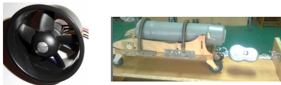
Fig. 10 EDF propulsion and test stand
