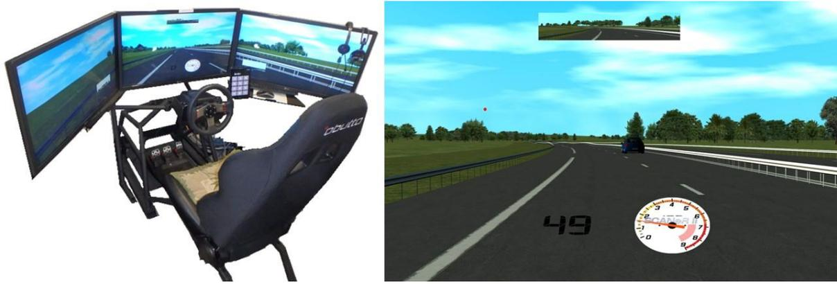
Figure 1. The left panel shows the driving simulator with the tablet device positioned next to the steering wheel. The right panel shows the central monitor view of the driving environment with rear-view mirror and digital speedometer displayed. A DRT target is presented above the horizon on the left.
