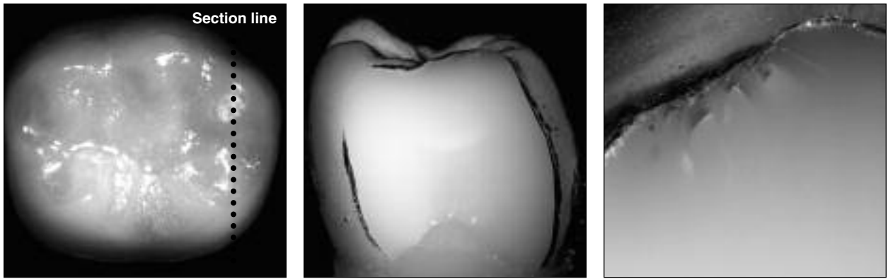
Fig 4 (left) Occlusal view and (center) cross section of an IPS e.max CAD crown at a load of 900 N exhibiting only minor occlusal damage (right) at 180,000 cycles after mouth-motion fatigue.
