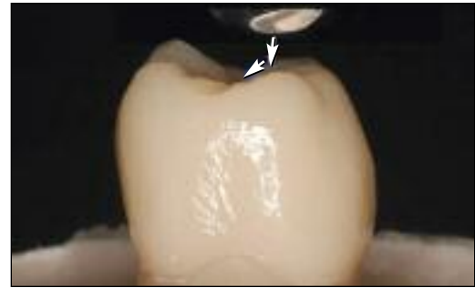
Fig 2 Mouth-motion fatigue with load application on the distobuccal cusp of the crown (arrows).
