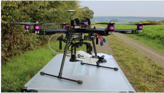
Fig.1: The used rotary-wing UAV with gimbal and mounted hyperspectral sensor Cubert UHD 185 Firefly.
