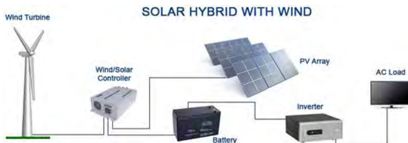
Fig. 4. Block diagram represent the structure of the hybrid system PV/Wind Hybrid System
