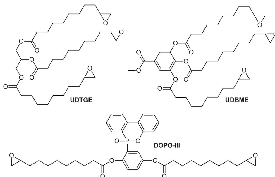
Fig. 5 Structures of epoxidized monomers used for resins.<sup>39,45,46</sup>
