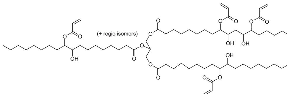
**Fig. 8** Acrylated epoxidized soybean oil monomers used for the preparation of fibre reinforced hybrid materials.<sup>57</sup>
