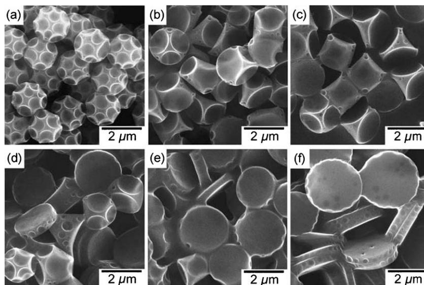
**Fig. 15** Scanning electron microscope photographs of PS/poly(lauryl methacrylate) (PLMA) composite particles produced by seeded dispersion polymerization in the presence of dodecane at various weight ratios of methanol/water media: a 80/20; b 82/18; c 84/16; d 86/14; e 88/12; f 90/10. (Reprinted with kind permission from Springer Science and Business Media from Ref. 84.)
