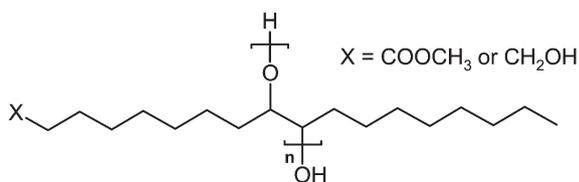
**Fig. 7** Polyols prepared by ring opening polymerization of epoxidized methyl oleate and subsequent partial reduction of the esters.<sup>52</sup>
