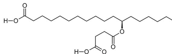
Fig. 10 12-Hydroxystearic acid succinate (HSAS) fatty acid derivative utilized to obtain biodegradable polymers with drug delivery application possibilities.<sup>69</sup>
