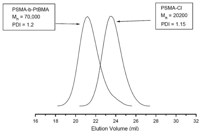
**Fig. 18** Size exclusion chromatography traces of a poly(stearyl methacrylate)-Cl macroinitiator and the resulting poly(stearyl methacrylate)-*b*-poly(*tert*-butyl methacrylate) diblock copolymer. (Reprinted with permission from Ref. 111, Copyright (2006), Elsevier.)
