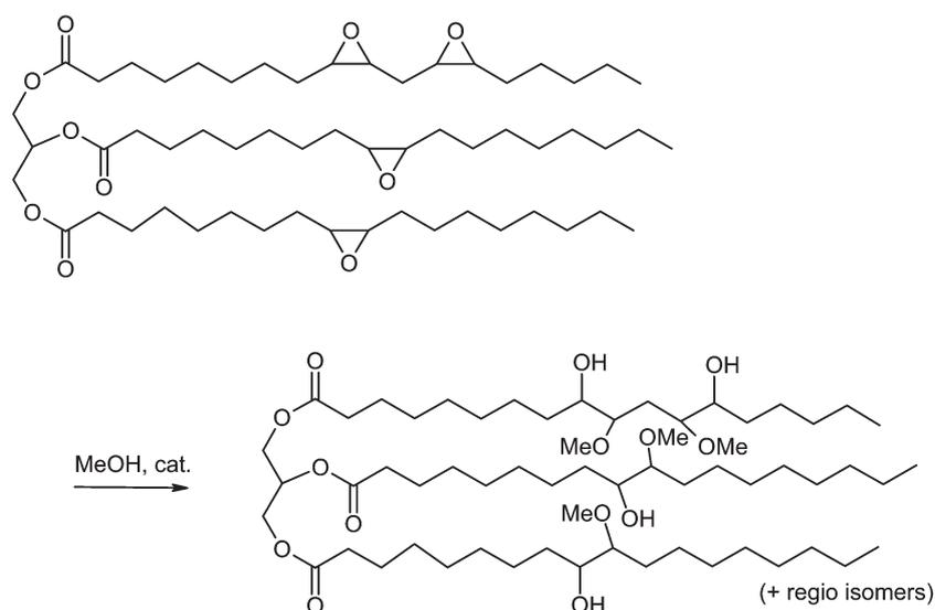
Fig. 6 Polyols prepared for polyurethane synthesis.<sup>49</sup>
