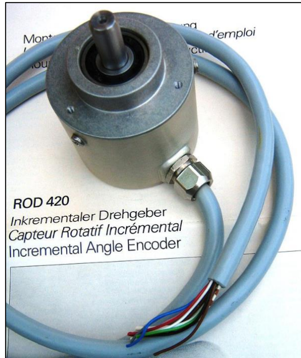
Figure 48. Incremental Rotary Encoder
