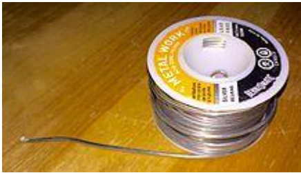
Figure 72. Spool of 1.6 mm Tin-Lead Solder
