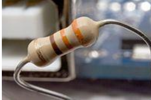
Figure 6. Typical Axial Lead Resistor
