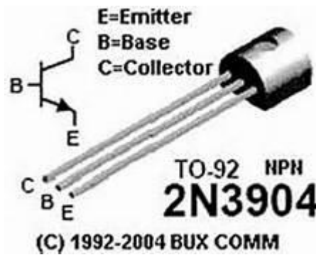
Figure 21. Typical BJT Appearance
