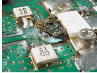
Power Transistor Failure
