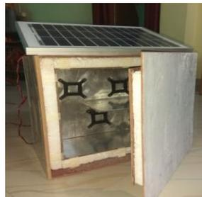
Figure: Construction of refrigerator
