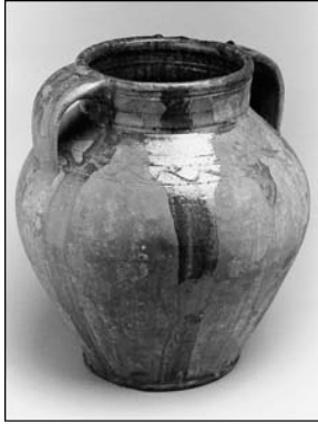
Figure 2: The ceramic pot in which the Kombucha tea was brewed. The glaze has visibly eroded from the internal and external surfaces of the pot.
