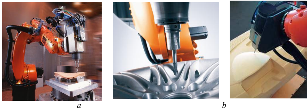
Fig. 1 - The processing of parts with Kuka robot help.[3],[ 7],[8].
