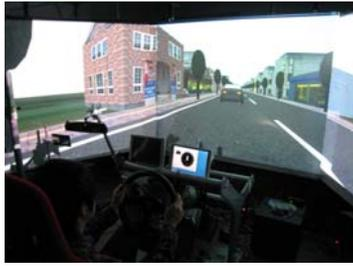
Fig.3 Front view of driving simulator
