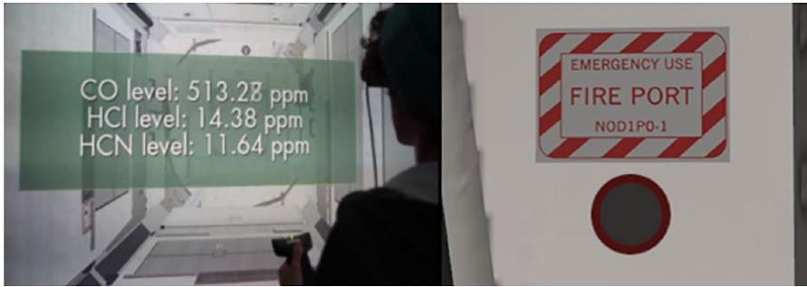
Figure 3. The Compound Specific Analyzer–Combustion Products (CSA-CP) in the virtual reality environment (VRE) displays environmental noxious gas readings (left) and fireport with identifier code (right).
