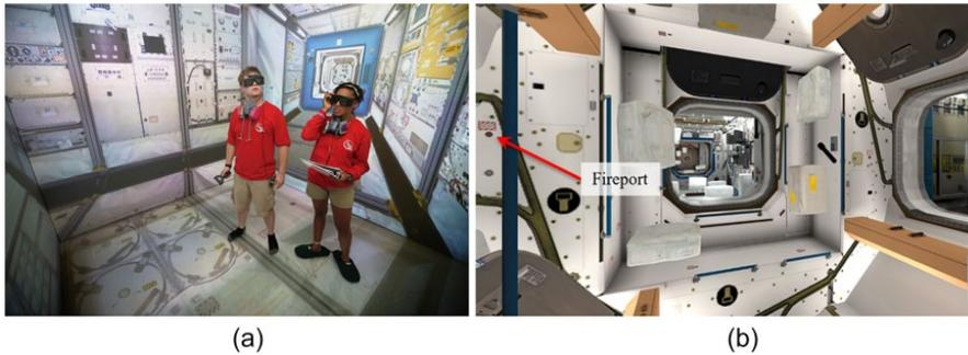
Figure 2. The (a) virtual reality International Space Station (VR-ISS) and (b) a fireport.
