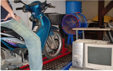
Fig. 2: Performance test on a dynamometer
