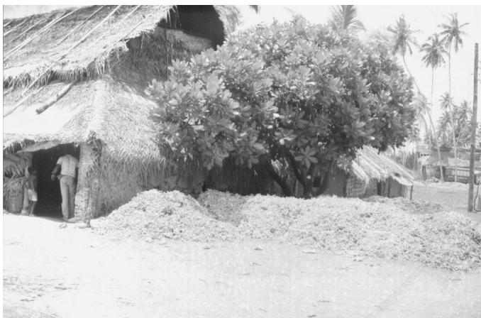
Fig. 4. Coral skeletons mined from nearshore reefs are burnt in kilns such as this one in Sri Lanka to produce lime for cement and building materials.
