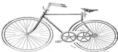
Fig -15: Gear Transmission Mechanism [14]
