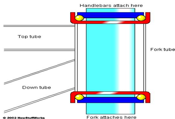
Fig -11: Fork Tube Attachments [11]
