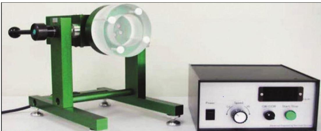
**Fig. 2. One axis clinostat with its control box in its horizontal rotation position**
