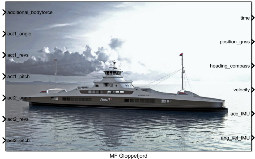
Figure 23: Simulink block for the VeSim interface
