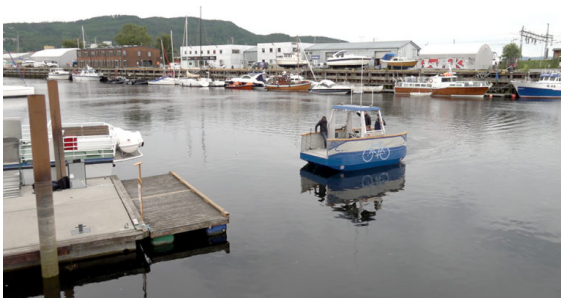
(a) The Autoferry prototype milliAmpere docking at Ravnkloa in Trondheim. Photo: Kai Dragland
