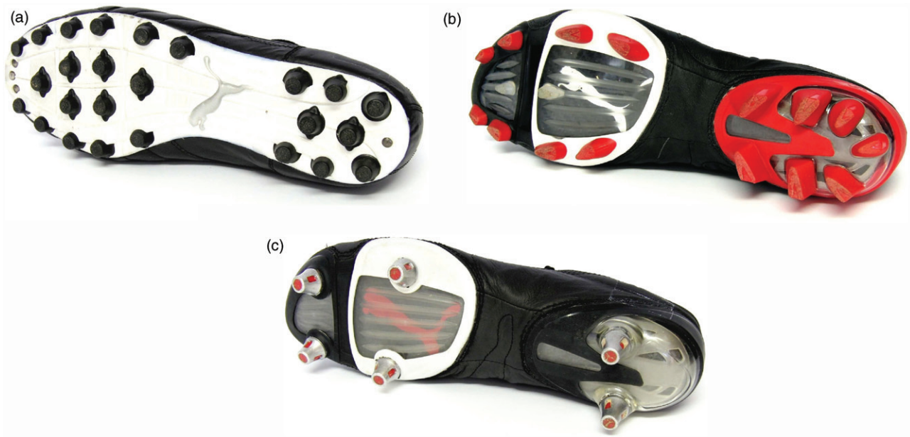
Figure 2. Shoe conditions: stud type (a) HG: hard ground, (b) FG: firm ground, (c) SG: soft ground.
