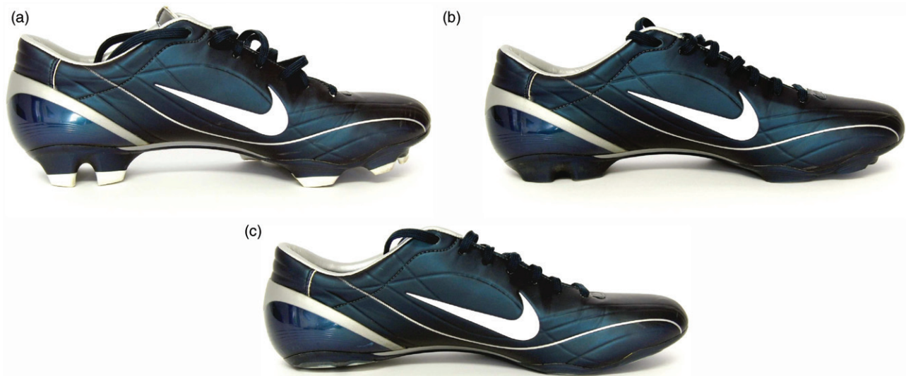
Figure 4. Shoe conditions: stud length (a) FFG: full firm ground with stud length 100%, (b) HFG: half firm ground with stud length 50%, (c) ZFG: zero firm ground with stud length 0%.
