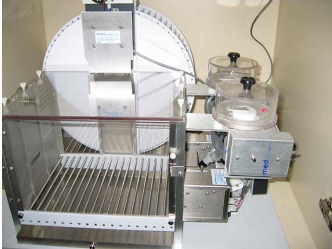
Figure 2-1. Photograph of the exercise chamber with running wheel attachment used for the exercise study. All rats regardless of group were placed in these chambers. A computer controlled master brake allows for the application of permanent brakes for the subjects in the non-exercise groups, or in the case of the exercise groups, the brakes are only engaged once the subject has reached its daily exercise limit of 56m.
