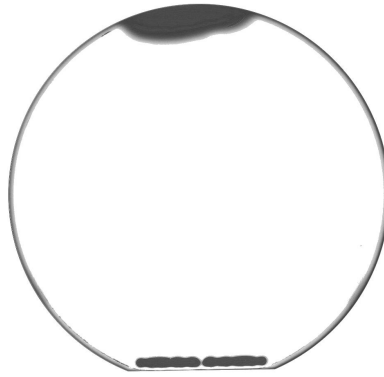
Fig. 7. SAM-picture of a bonded silicon wafer using a 133nm BCB layer. The picture shows no defects in the bond interface. The black part on the upper side of the wafer results from the delamination by the razor blade test, done before the SAM investigation. Delamination at the bottom is caused by the wafer label.
