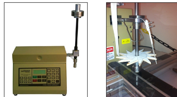
Figure 3: Abrasion tester, which was adapted to perform rotating movements instead of linear movements by using a gear wheel (right)
