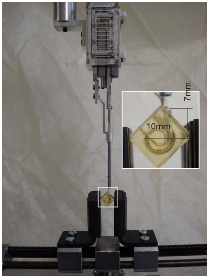
Fig. 11. Experimental setup for experiments using the Insertion Tool to insert an electrode array into a cochlea anatomical model.
