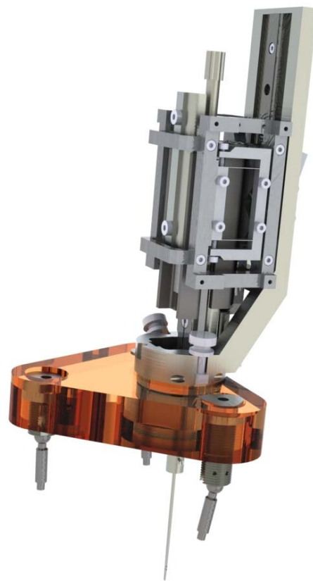
Fig. 14. CAD Drawing of the Automated Insertion Tool we describe in this paper as we envision it being integrated to the Microstereotactic Table developed by Labadie et. al. [9], which we envision providing a means of accurately positioning the insertion tool under image guidance.
