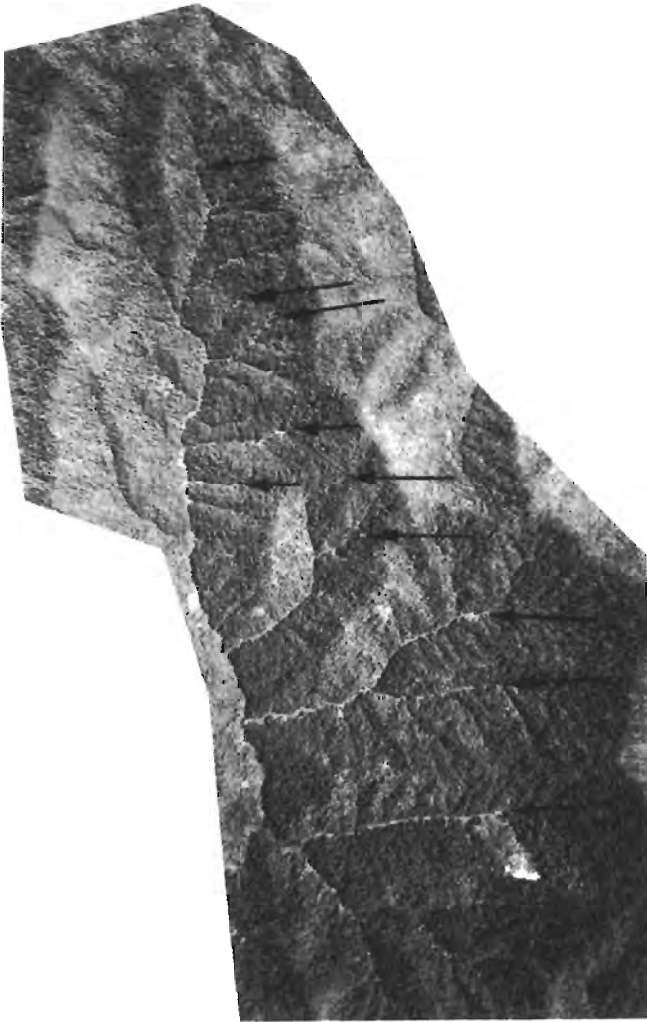
FIGURE 11.1. Aerial photograph taken in 1939 of a 4th-order basin in the western Olympic Mountains, Washington. The storm of record (1934) triggered numerous debris flows (indicated by arrows) that deposited into the main channel. Orme (1990) and
