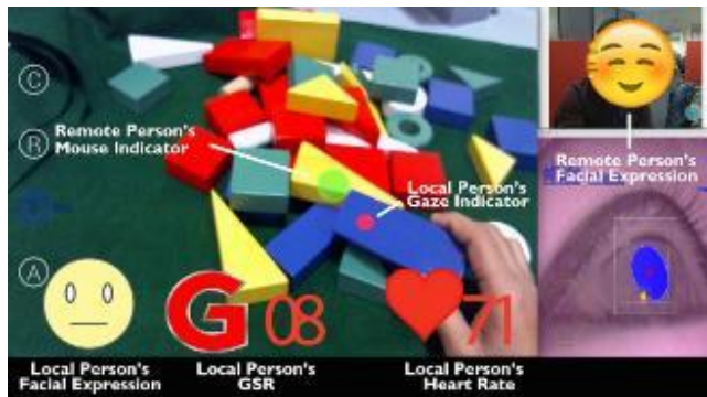
Fig. 6. Remote helper’s screen view showing local worker’s workspace, gaze, emotions (facial expression), heart rate, and GSR in real-time [5].
