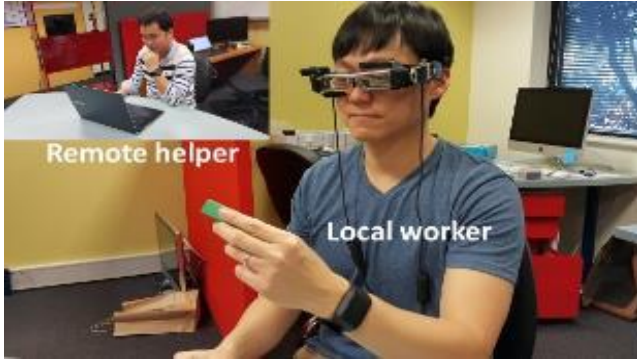
Fig. 5. A local worker wearing Empathic Glasses and a remote helper using a desktop computer [6].
