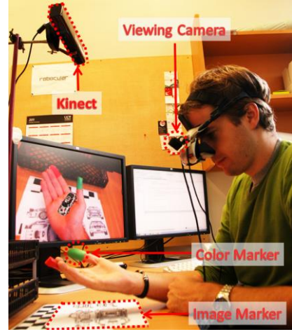
Figure 3: The interaction set up. The Kinect is suspended above the interaction volume, with the reference image marker below it.
