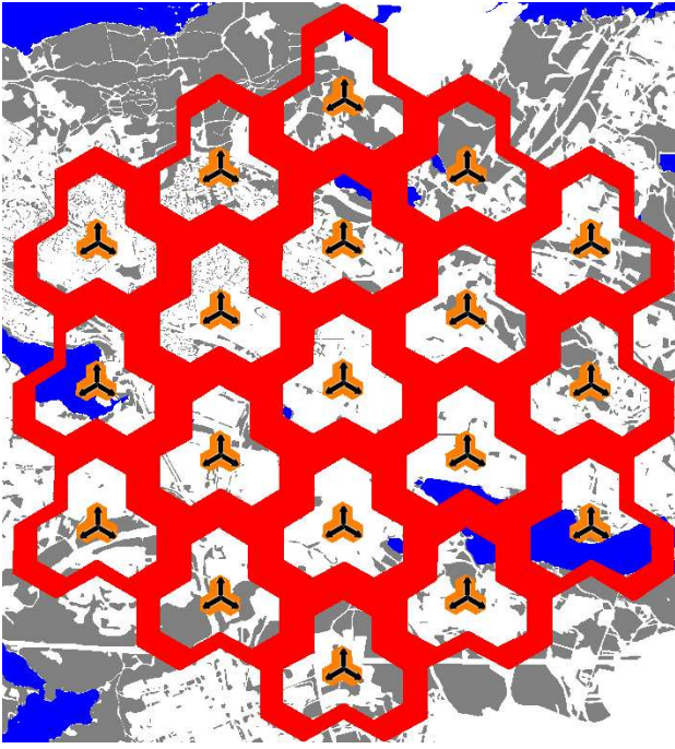
Fig. 2. Illustration of the traffic distribution into smaller hexagons close to the base stations and of the traffic distribution at the edges of hexagons.
