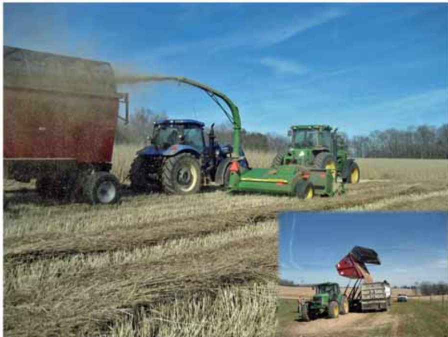
Fig. 2.4 Field chopping “pre-processes” switchgrass, producing a flowable material that is easier to handle by the process systems within a biorefinery. However, such systems require additional labor to collect the chopped material in the field and haul to a central collection point (as in the insert) and specialized storage.
