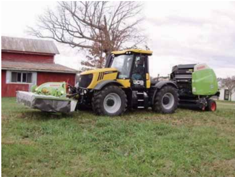
Fig. 2.5 A combined mower and baler designed for one-pass harvesting of herbaceous biomass such as switchgrass. Such systems will reduce labor required to harvest and bundle biomass.
