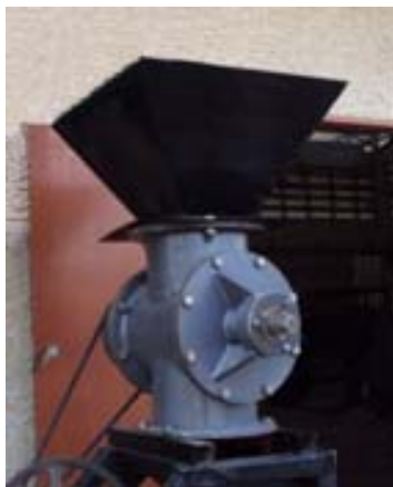
Figure 2: The rotary airlock valve developed
