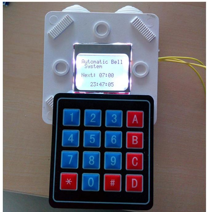
Fig. 3. Real time actuator node prototype
