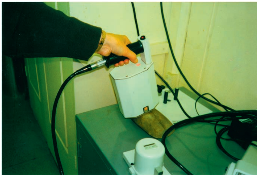
Figure 8.2 Portable XRF being used to measure a stone axe in the Ashmolean Museum, UK. The axe is too large and heavy to place on the instrument aperture, so the probe is held against one side of the axe. Reproduced with permission from the Ashmolean Museum.
