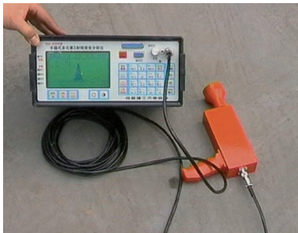
Figure 7.2 IED-2000P PXRF analyzer which incorporates a Si-PIN detector.
