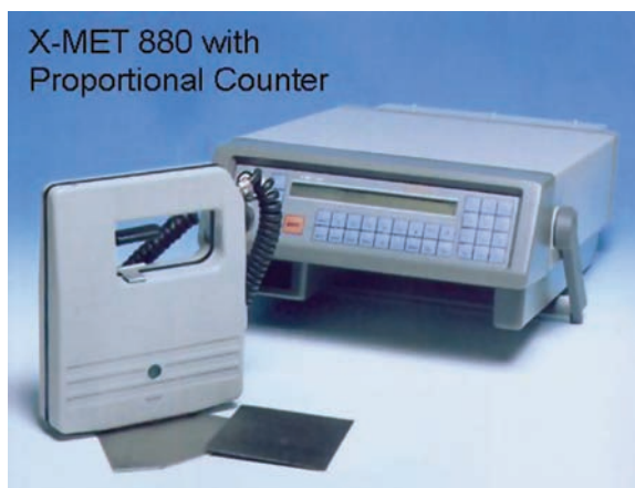
Figure 6.11 Portable XRF analyser with gas-filled proportional detector. Note the two separate modules, probe and electronic unit. The total weight of the system was about 8 kg. Introduced in 1984 by Metorex Inc., it was manufactured for over 12 years. The LCD display is just two lines by 40 characters each.
