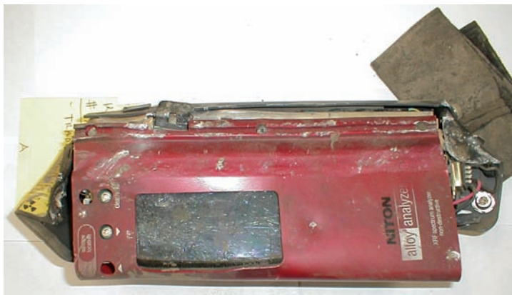
Figure 6.16 An older Model XL 800 with radioisotope sources, apparently run over by some heavy equipment. The left end of the instrument houses radioisotopes, which survived the accident.
