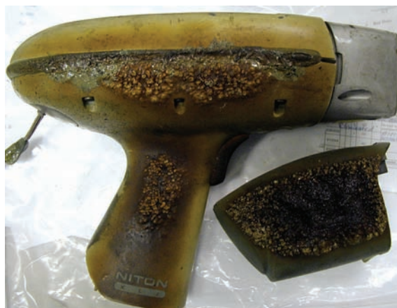
Figure 6.15 Model XLt 800 with miniature X-ray tube after damage in fire.
