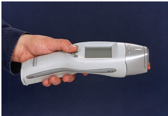
Figure 6.14 Modern, handheld XRF analyser with “p-i-n” diode silicon detector and isotope excitation. This unit can incorporate up to three different isotopes for increased elemental range.
