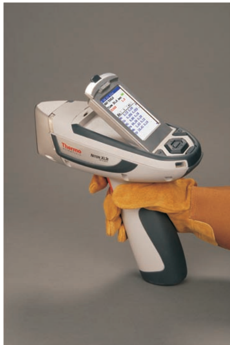
Figure 6.13 Modern, handheld XRF analyser with “p-i-n” diode silicon detector. This single piece unit with miniature X-ray tube weighs less than 1.4 kg. The photograph shows the latest model of the analyzer – its predecessor was originally introduced to market in the spring of 2002. Tilted, LCD touch screen is 1/4 VGA in size.
