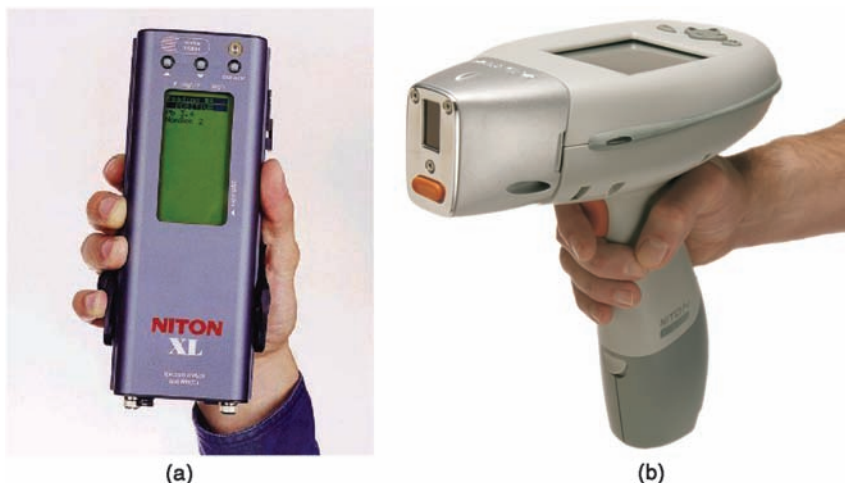
Figure 4.9 Niton Models XL-300 (a) and XLp-300 (b) Series Lead in Paint Analyzers.
