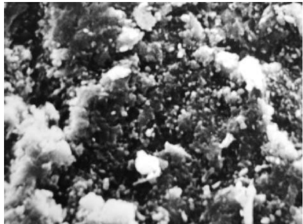
Figure-7: SEM picture of the reaction product of Al 2 O 3 -NaCl system (molar ration 1:1), oxidized at
