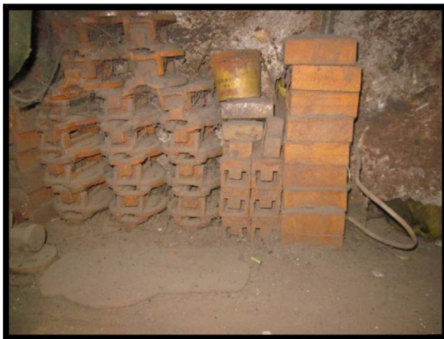
Plate 5. Inventories lying on floor covered with layers of rust
