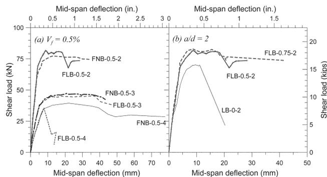
Fig. 3—Shear load-deflection relationship.
