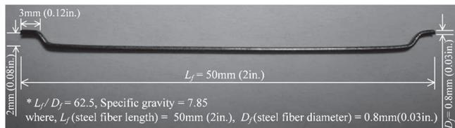
Fig. 2—Dimension for hooked steel fiber.
