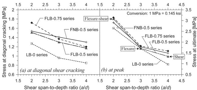
Fig. 6—Measured average shear stresses versus  $a/d$ .
