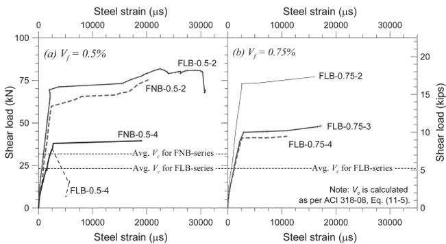
Fig. 5—Shear load-bar strain relationship.
