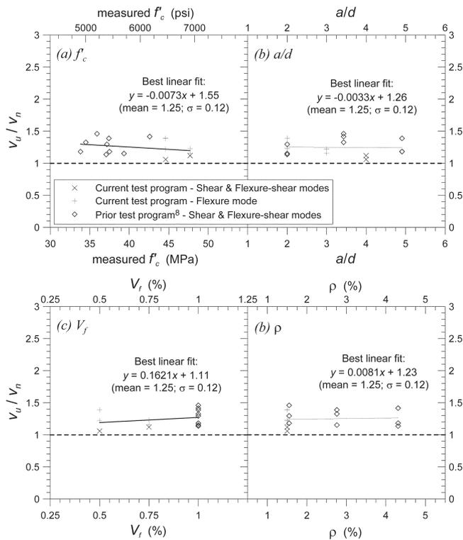
Fig. 7—Ratio of measured average shear stress at peak to shear stress  $v_u/v_n$  calculated based on design shear strength model developed for SFRLC beams (Eq. (1) and (2)).
