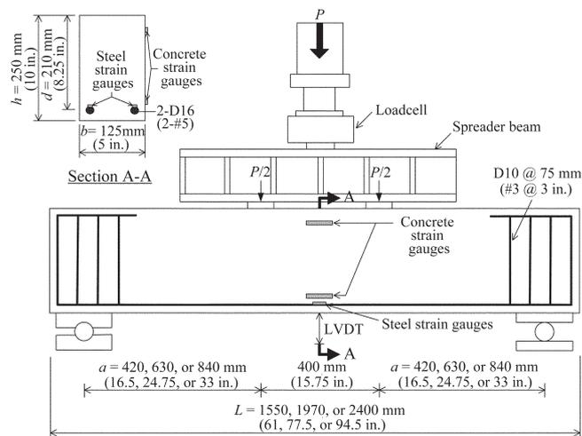
Fig. 1—Test setup and tested beam (not scaled).
