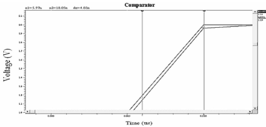
**Figure 5:** Results for slew rate of Comparator.
