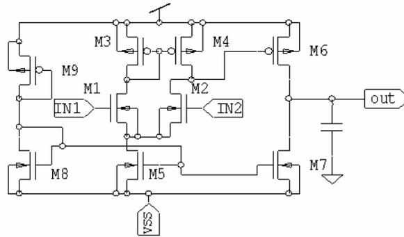
**Figure 1:** Proposed design of a CMOS comparator.
