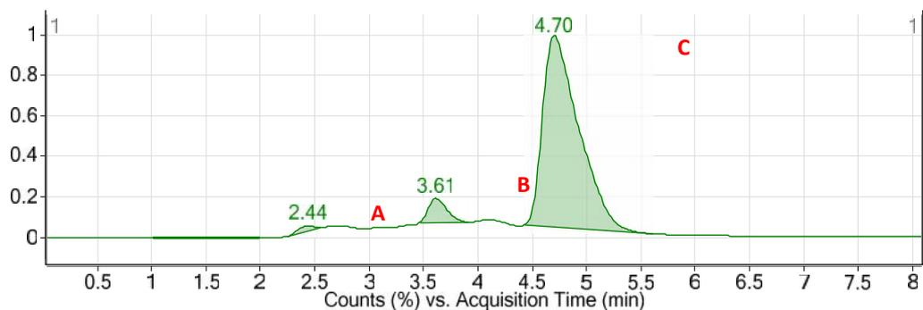
**Figure 3: EIC Representative HPLC elution profile of (A) Cephalixin, (B) Amoxicillin and (C) Ampicillin standard**
