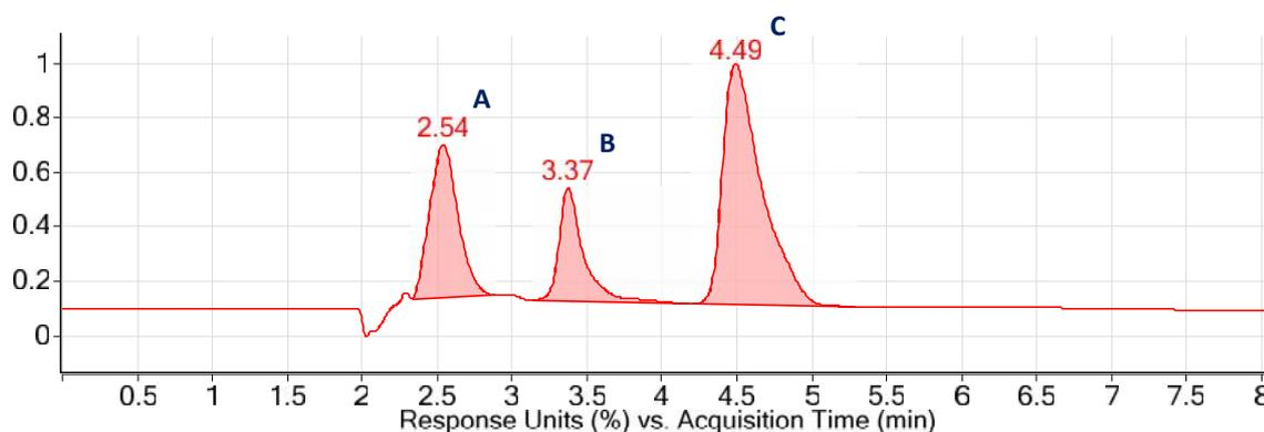
**Figure 2: DAD Representative HPLC elution profile of (A) Cephalexin, (B) Amoxicillin and (C) Ampicillin standard recorded at 257 nm is shown.**
