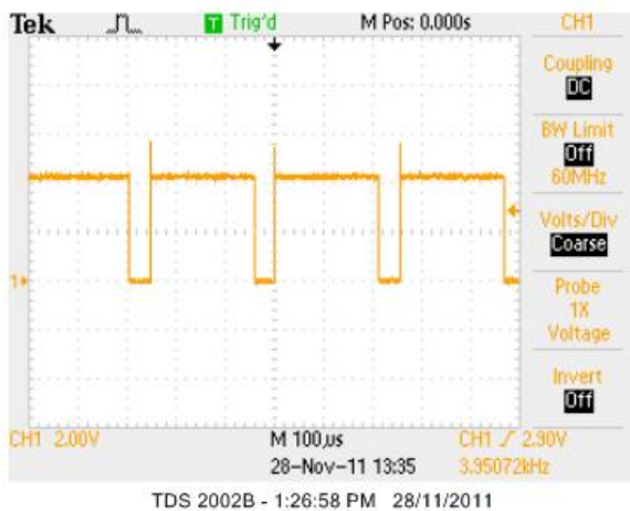
Figure 7: Reading from 555 timer when the cuff is at rest
