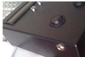
Figure 6: Design of the outer casing for the occlusion cuff, showing the power adaptor input
