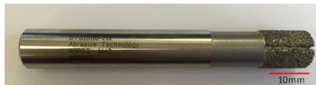
Figure 9. Unused diamond bonded 10 mm diameter end mill.
