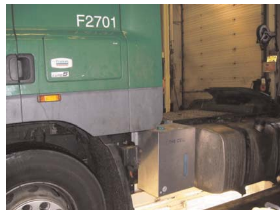
Figure 4. The hydrogen generator is the box in front of the diesel fuel tank.
