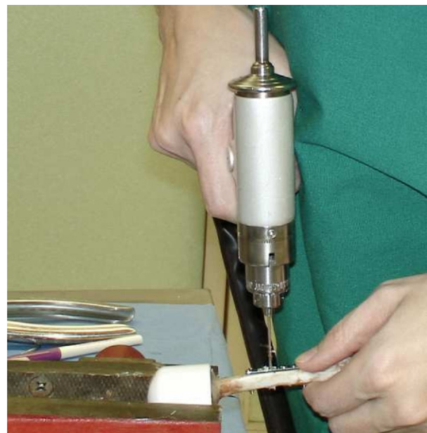
Figure 1. Screw holes were predrilled in all rabbit femurs with a 1.5-mm drill bit and air drill and then tapped before placing 2.0-mm bone screws by hand to hold the 2.0-mm plate to bone. Predrilling and tapping decrease local stress, lessening the likelihood of traumatizing the bone.
