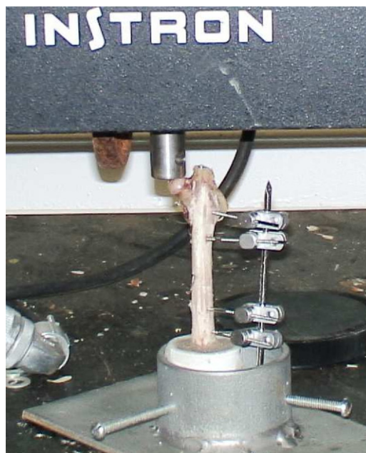
Figure 3. The Instron Model 4201 machine is specifically designed to simulate the natural stresses that occur on bones in live animals. It then records the maximum amount of pressure that can be applied before either the bone or the implant fails.
