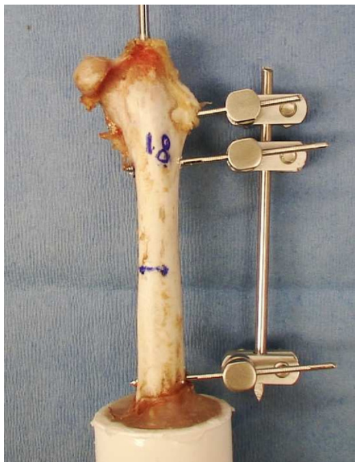
Figure 2. Typical construct placed on rabbit femurs of 3/32" IM pin and ESF with 1.57-mm or 0.062-inch mini half pins with positive profile threads tied into a 1/8" fixation bar with single mini SK clamps. Bones repaired with this method withstood an average of 67 lb (91 N) of bending and compressive forces before the bone (not the fixation device) failed.
