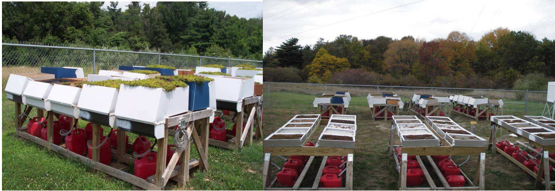
Figure 2. Green roof experiments (left, growing media depth experiment in built-in-place models; right, different growth media formulations in Green Roof Blocks™) at the Environmental Sciences Field Site at Southern Illinois University Edwardsville. Each green roof model has a separate storm water collection system so that storm water runoff quantity and quality can be evaluated for each individual system.
