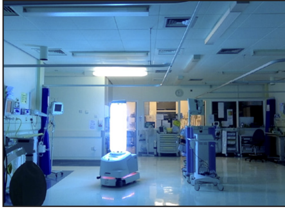
Fig. 13 UVD Robot can be programmed to cover large area with UV sterilization, but only after staff members have exited for safety.
