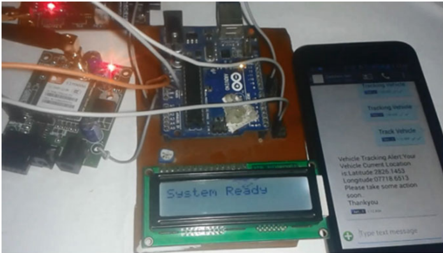
Fig. 4 Hardware setup of GPS-GSM-based marine monitoring system
