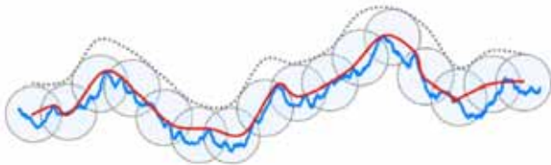
Picture 11. Morphological opening filter (upper red curve) obtained by rolling a disk over the profile [5]
