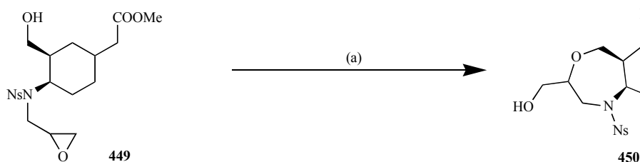
Scheme 87. Synthesis of oxazepane ring by ring-opening/ring-closing of epoxide ring. Reagents: BF 3 ·OEt 2 , CH 2 Cl 2 , rt, 2h [269].
