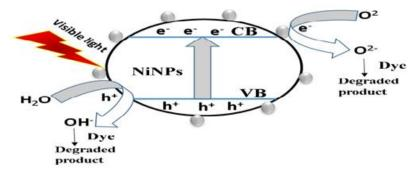
Figure 7: Mechanism of dye removal by nickel nanoparticle in dye sensitized solar cells<sup>108</sup>.
