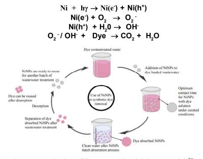
Figure 6: Mechanism of dye removal by nickel nanoparticle<sup>94</sup>.
