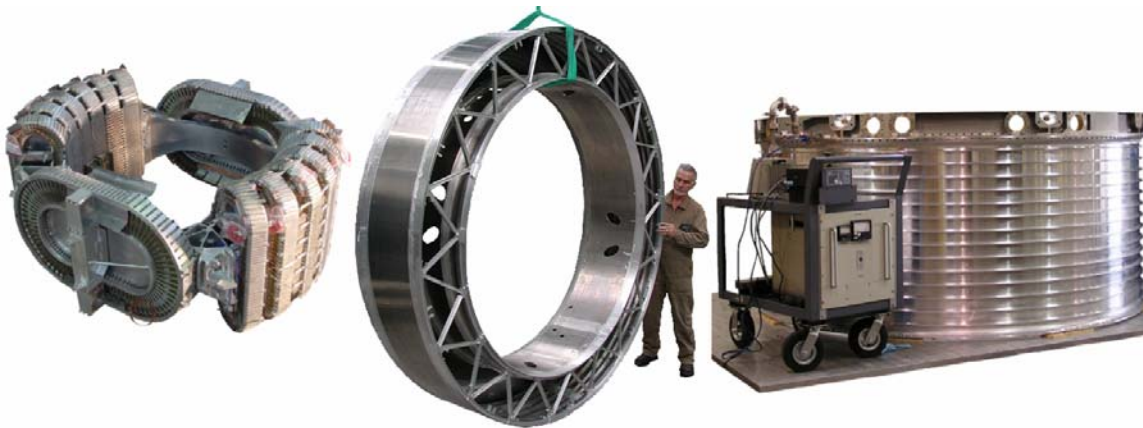
Figure 2. Photographs of the assembled magnet coils, the lower half of a helium vessel, and the vacuum vessel during manufacture in England, Switzerland and the USA.
