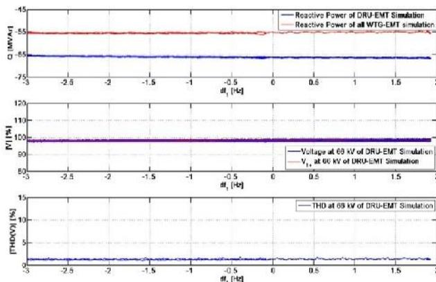
Fig. 13 System with B12 DRUs investigated with detailed cable string model. Depicted Q, V and THD.
