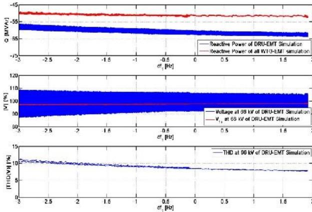
Fig. 12 System with B6 DRUs investigated with detailed cable string model. Depicted Q, V and THD.
